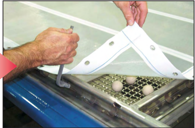
Steel Top Cover and Screen Frame Construction
